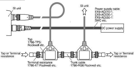
\* SMC only provides the SI unit and the power cable. Please refer to other manufactures for additional parts needed.
