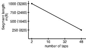
Allowable maximum length of segment = 1000m (3280feet) - 16.3m (53.4 feet) x [number of tap - 2]
