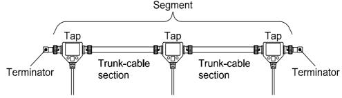
The total allowable length of a segment depends upon the number of taps in your segment. There is no minimum trunk-cable section length requirement. The maximum allowable total length of a segment is 1,000m (3,280ft.) with two taps connected. Each additional tap decreases the maximum length of the segment by 16.3m (53ft). The maximum number of taps allowed on a segment is 48 with a maximum length of 250m (820ft.).
