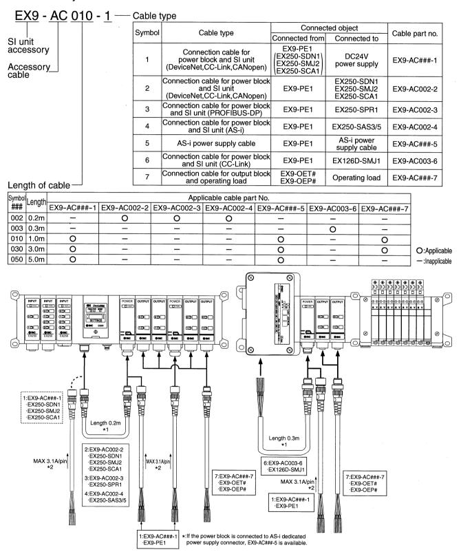
\*1: This cable is a bypass cable used for the layout where the power block is located to the right of the SI unit. \*2: If max. supply current (3.0 to 3.1A) is applied for operation, do not make the ambient temperature exceed 40°C and bundle the cable. Note: The cable and the power block allow the current up to 3.1A\*<sup>2</sup>.
