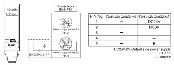
B.The supply of power from the power block connector to the SI unit
