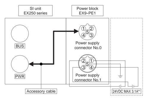
\*1:If max. supply current (3.0 to 3.1A) is applied for operation, do not make the ambient temperature exceed 40°C and bundle the cable.
