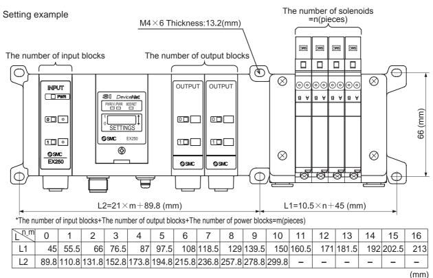
\*Each dimension is for the condition with VQC1000 series solenoid valve and EX250 series connected. With regards to the dimension L2, the standard setting is what makes the relation, m≦10. For setting of pieces over 10, consult with SMC sales.
