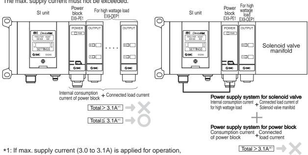
do not make the ambient temperature exceed 40°C and bundle the cable.
