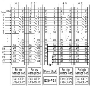
Fig. Connector wiring between output blocks
