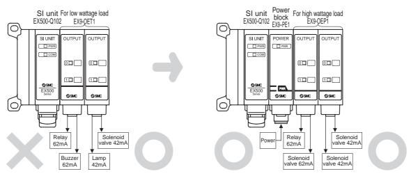
(5)The number of output point when the power block is used
