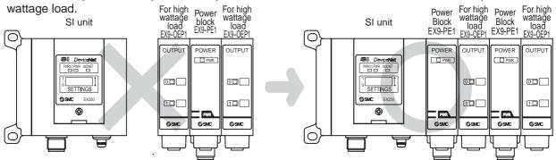
(3)Output block for low wattage load
