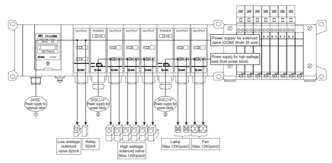
Fig. Power supply system diagram for output block
