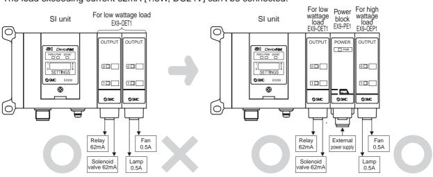
EX126/EX250 series (except for one power supply system of AS-i) The load exceeding current 62mA [1.5W, DC24V] can't be connected.
