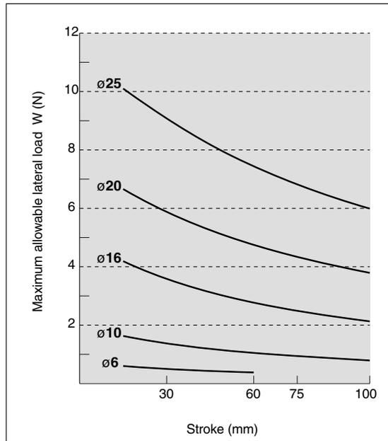
Note 1) The allowable lateral load varies depending on the size of a load (the distance to the load's center of gravity). Please contact SMC for further details.
