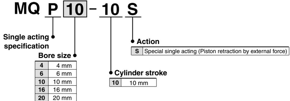
\* The MQP series is not auto switch capable.
