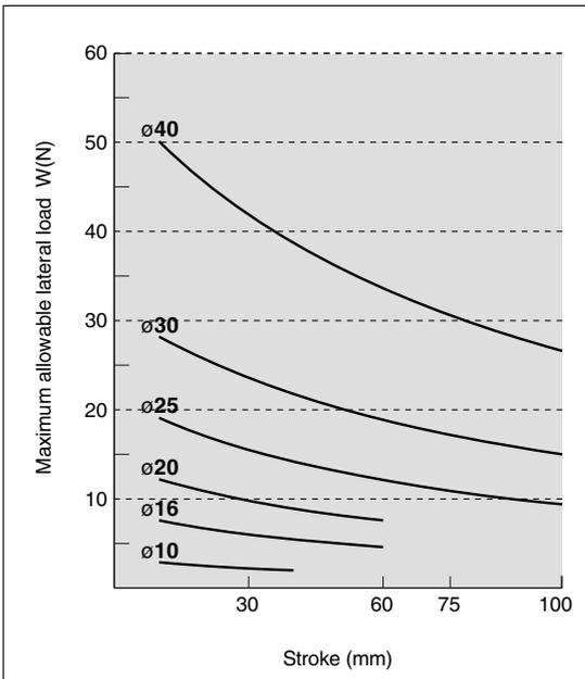
Note 1) The indicated allowable lateral load at the rod end is for the rod end female thread.
