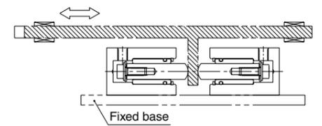
Using two MQP cylinders can improve the thrusting accuracy of an MQQ and/or MQM double acting metal cylinder. Additionally, equal strength of both extension and retracting thrust can be obtained.
