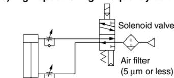
\* When using a solenoid valve, use a metal seal type (Series VQ, VQZ, SQ, etc.).
