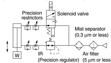
\* When using a solenoid valve, use a metal seal type (Series VQ, VQZ, SQ, etc.).
