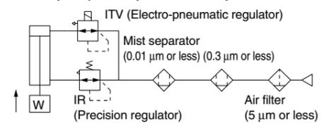
\* When performing control of cylinder output, do not create a restriction circuit using a speed controller, etc. Pressure inside the cylinder will drop and control will become impossible. Always control actuation by means of pressure control.
