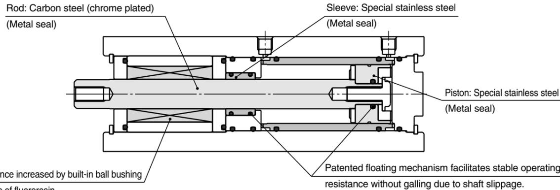
Lateral load resistance increased by built-in ball bushing
