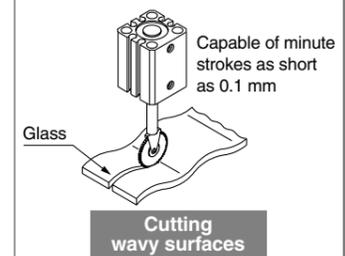
Tension controlling responding to very low pressure and minute pressure variations
