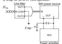
5. If the feed back circuit of the VEA252 will not be used, insert jumper pin J1 on the board on the "1" side. This will disable the feedback circuit, and the VEA252 will assume the same function as that of the VEA251.
