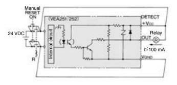
If a short circuit occurs at the current output terminal side, the power supply is shut off immediately to prevent damage to the output circuit of the power amplifier. The manual  $^{\mbox{\scriptsize RESET}}_{\mbox{\scriptsize ON}}$  switch is to be pressed to start or restart.
