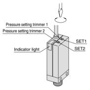
Set the possible min. pressure for adsorption confirmation. If setting the pressure lower than that, switch becomes ON in case that adsorption is not completely done. If setting the pressure higher than that, switch does not become ON even though it may absorb workpieces.
