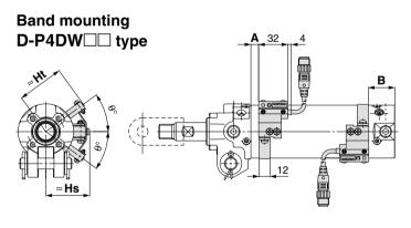
Note) The above drawing is the switch band mounting example for the D-P4DWS  $\!\Box$  type.
