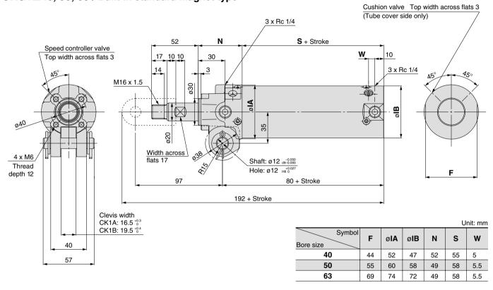
CKG1□40, 50, 63 / Example: Built-in standard magnet type + Magnetic field resistant auto switch D-P4DW□□ type (Band mounting)
