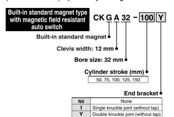
Note) Knuckle pin, cotter pin and flat washer are provided as a standard for Y.
