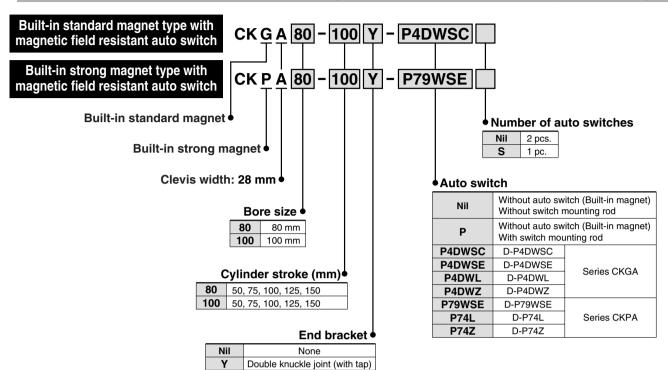
Note) Knuckle pin, cotter pin and flat washer are provided as a standard for Y.
