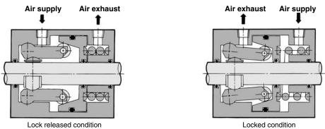
Brake piston is operated by air pressure and spring force.
