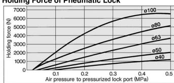
**Holding Force of Spring and Pneumatic Lock**
