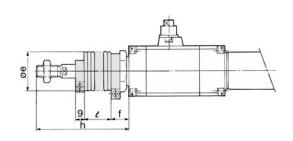
(mm) Bore Stroke range AL Вı B2 ВС BN BP BQ BZ Ε GΑ GB GC GD GK GL GQ GR H1 H<sub>2</sub> 20\_0.033 20 to 300 18 15.5 13 26 38 80 1/8 1/8 57.5 8 13 73.5 8 8 55 3.5 6 4 4 41 5 8 28 1/8 1/8 26\_0.033 25 to 300 19.5 17 32 45 90 69 10 13 83.5 8 9 64.5 4 9 7 7 45 6 8 33.5 1/8 1/8 69 26\_0.033 32 to 300 22 19.5 17 32 45 90 12 13 83.5 8 9 64.5 4 9 7 7 45 6 8 37.5 32\_0.039 90.5 21 41 52 100.5 1/8 1/8 76 14 16 8 4 50 8 10 46.5 40 to 300 22 11 70 11 8 7
