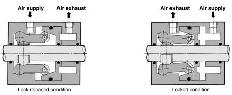
Brake piston is operated by air pressure.
