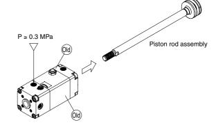
4) Similarly, apply 0.3 MPa or more of compressed air to the unlocking port of the new lock unit, and replace the new lock unit's temporary axis with the previous piston rod assembly.
