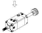
5) Reassemble in reverse order from steps 2) and 1). When retightening the sections, turn approximately 2° past their position prior to disassembly.
