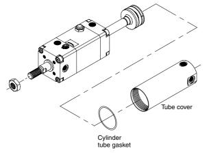
Apply 0.3 MPa or more of compressed air to the unlocking port, and pull out the piston rod assembly.
