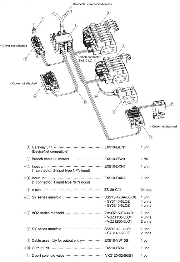
\* Two branch connectors are attached to the manifold including the SI unit and two are attached to the input unit and the output unit respectively. The branch connector (EX510-LC1) is used to connect the individual units.
