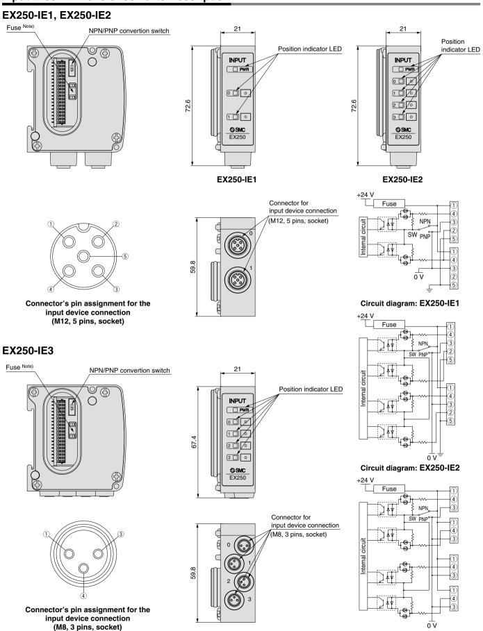
Note) Fuse for overcurrent protection If addressing the possible cause of a problem, even when the fuse is blown, it can be reinstated by replacing with a fuse as shown in options, page 1673.
