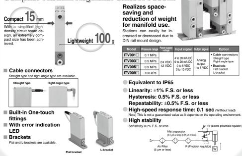
Electro-Pneumatic Regulator Series ITV1000/2000/3000 Electronic Vacuum Regulator Series ITV209
