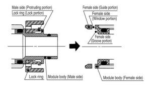
2. By inserting the lock ring, the lock portion touches female side guide portion and falls into the direction shown with the arrow.
