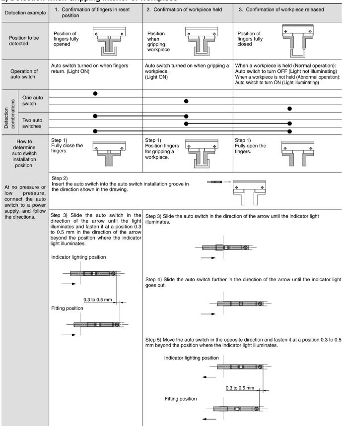
Note 1) It is recommended that gripping of a workpiece be performed close to the center of the finger stroke.
