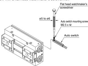
Note) Use a watchmaker's screwdriver with a grip diameter of 5 to 6 mm to tighten the auto switch mounting screw. The tightening torque should be about 0.05 to 0.15 N·m.
