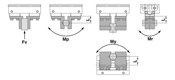
L: Distance to the point at which the load is applied (mm)
