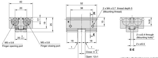
\* Use the attached hexagon socket head screws for mounting holes.
