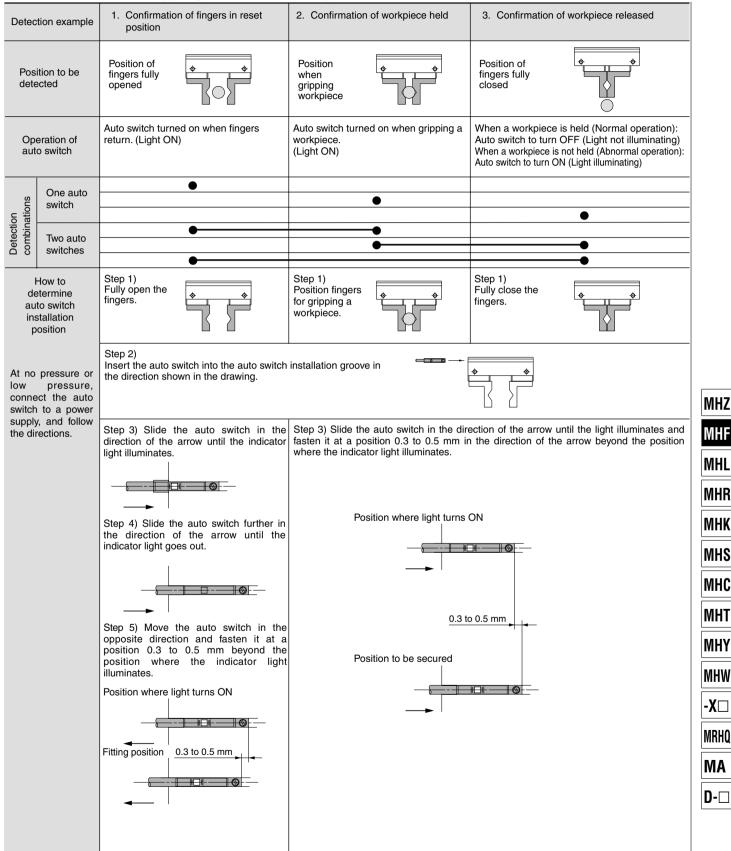
Note 1) It is recommended that gripping of a workpiece be performed close to the center of the finger stroke.
