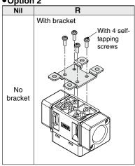
Note) Each option is not assembled with the product, but shipped together. If an accessory is required, order separately using "ZS" part numbers.
