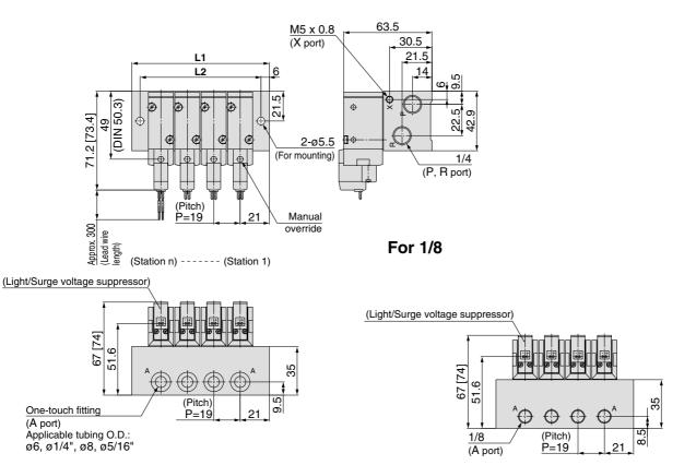
L plug connector (L) M plug connector (M)
