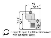
Type 42 Manifold: Side Ported (Pilot valve is on the A port side)/SS3YJ3-S42-Stations -M5, N3
