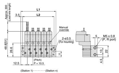
Type 41 manifold: Side ported / 10-SS3YJ3-41- Station - M3
