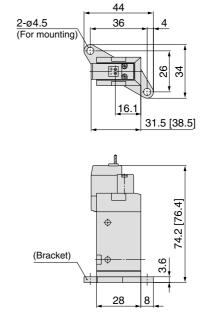
L plug connector (L): SYJ7□2-□L□□-01□ (-F) M plug connector (M): SYJ7□2-□M□□-01□ (-F)
