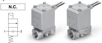
When the valve is closed, flow is blocked from port 1 to port 2. However, if the pressure in port 2 is higher than port 1, the valve will not be able to block the fluid and it will flow from port 2 to port 1.
