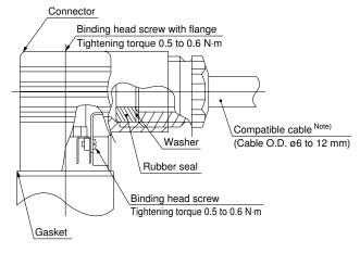
Note) For an outside cable diameter of ø9 to 12 mm, remove the internal parts of the rubber seal before using.
