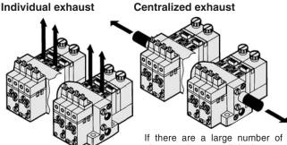
If there are a large number of ejectors that are linked on a manifold and operate simultaneously, use the builtin silencer type or the port exhaust type.
