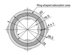
**ZPT1-A5** is a recommended adapter. (Four adapters are necessary.)
