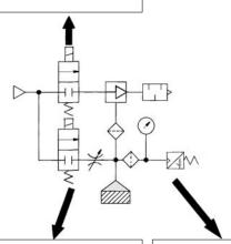
Select a vacuum switching valve that has a conductance that does not reduce the composite conductance consisting of the areas from the pad to the ejector.
