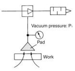
**Exercise:** Using a supply pressure of 0.45 MPa, when the ejector (ZH07□S) picks up a workpiece that leaks air, the vacuum gauge indicated a pressure of −53 kPa. Calculate the leakage volume from the workpiece.
