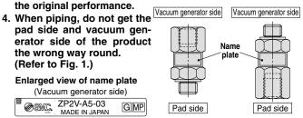
Fig. 1. Mounting direction
