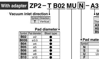
\* Blast type: Work pieces can be removed easily.
