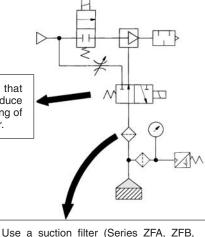
For the release valve, select a 2/3 port valve with a low vacuum specification. Also, use a needle valve to regulate the release flow rate.
