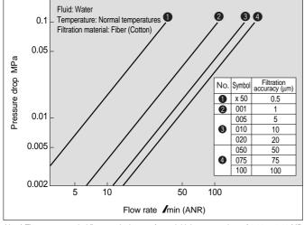
Note) The recommended flow rate is the rate for an initial pressure drop of 0.01 to 0.02 MPa.
