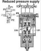
When the pilot solenoid valve "a" is energized (or when pilot pressure is applied to the port P1 of the air operated type) while the port P1 is under the pilot pressure, reduced pressure is supplied from the port 3 (R) to the port 2 (A).
