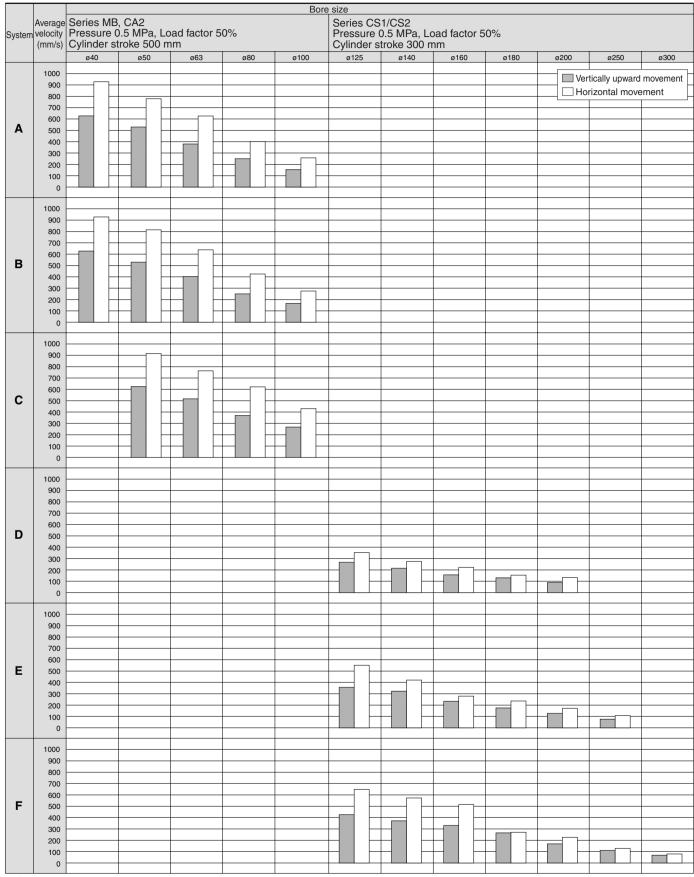
\* When the cylinder is extended, the speed controller is metered-out, is connected with the cylinder directly, and its needle is fully open. \* Values on the average velocity of a cylinder are obtained from the stroke length divided by full stroke time.
