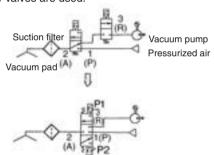
•There is no blow-by when switched from vacuum suction to vacuum release or vice versa.
