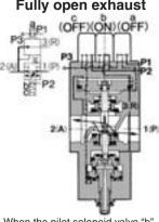
When the pilot solenoid valve "b" is energized while pilot pressure is in the port P2 (or when the pilot pressure is applied to the port P2 of the air operated type), an acting force generated above the operation piston (and pushes down the operation piston, and thus the ports 1 (P) and 2 (A) are connected.
