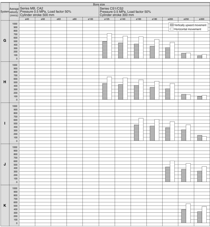
\* When the cylinder is extended, the speed controller is metered-out, is connected with the cylinder directly, and its needle is fully open.
