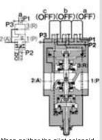
When neither the pilot solenoid valve "a" nor "b" is energized (or when no pilot pressure is applied to the ports P1 and P2 of the air operated type), no acting force is applied to the pressure control piston (a) and operation piston (b), and the spring (c) closes both poppet valves (a), thus the valve assumes the closed center procition.
