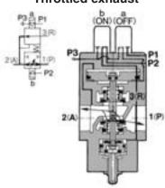
When the pilot solenoid valve "b" is energized while pilot pressure is in the port P2 (or when the pilot pressure is applied to the port P2 of the air operated type), an acting force generated above the operation piston (§) pushes the operation piston down, and thus the port 1 (P) and port 2 (A) are connected.
