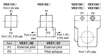
Note 1) Port P2 is not compatible with VEX1□00. Note 2) A Silencer is mounted to port P2 for VEX1□01 as a standard. For the 2 steps directional control and multiple steps pressure control setting, use the product after removing a silencer.
