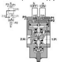
When the pilot solenoid valve "a" is energized (or when pilot pressure is applied to the port P1 of the air operated type) while the port P1 is under the pilot pressure, reduced pressure is supplied from the port 3 (R) to the port 2 (A). The acting force of the pilot pressure (port P1) reaches the space under the pressure control piston ③ pushes the piston upward and opens the poppet valve ⑥. Thus air is supplied from the port 3 (R) to the port 2 (A).
