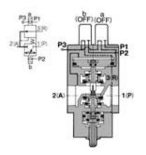
When neither the pilot solenoid valves "a" or "b" is energized (or when no pilot pressure is applied to the ports P1 and P2 of the air operated type), no acting force is applied to the pressure control piston (a) and operation piston (b), and the spring (c) closes both poppet valves (c), thus the valves assume the closed center position.
