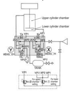
The two economy valves (hereinafter called VEX)  $\bigotimes$  and  $\bigotimes$  and a tank composes a main system that drives the double acting cylinder, and the small regulator (hereinafter called REG) and pilot valve (hereinafter called SOL) remote control the economy valve.
