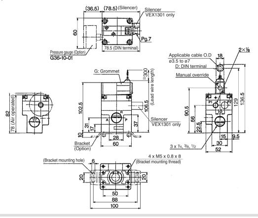
Air operated: VEX1500 External pilot solenoid: VEX1501
